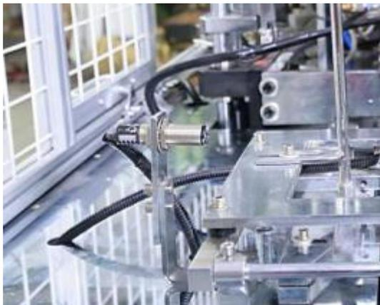
Encoder and the sensor control the machine at the same time, one paper fan match one bottom, no waste.
