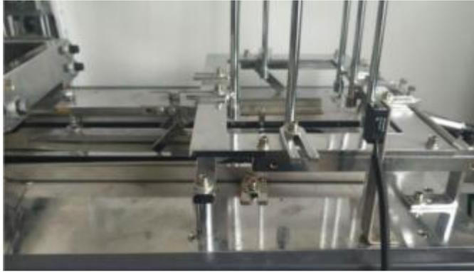
Paper can be well adjusted with three times feeding process, avoid the irregularity during folding paper fan.
