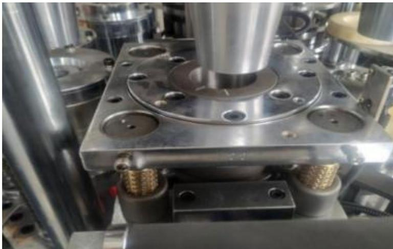
When give the bottom paper, sometimes the bottom paper will be turned over, cannot match the paper fan well, this machine shorten the process, give bottom directly, avoid the problem.
