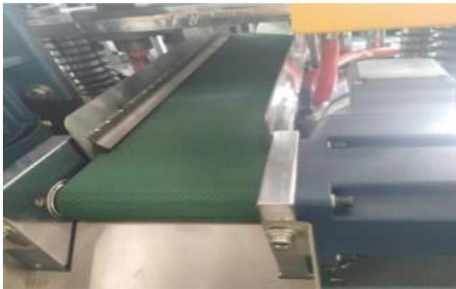
Waste paper discharged by the tube. When the machine working, avoid the waste paper enter the machine inside part, affect machine running.
