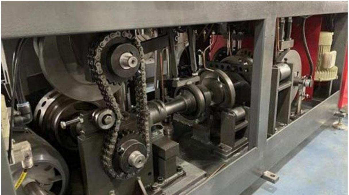
Disposable paper cup machine It has over-cup detection, cup-tube forming detection, and automatic shutdown alarm for faults. The process flow of the equipment is as follows:
